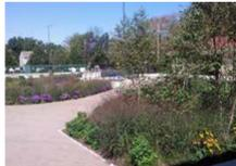
The area is suitable for a rain garden. A rain garden is planted with specially selected plant species that collects stormwater from hard surfaces and allows that rainwater to infiltrate into the ground, evaporate, or be absorbed by the plants.
